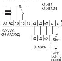
The terminal voltage of evaluation units ASW454 or ASW454/24 can also be checked with a voltmeter between the "a2" and "a3"
