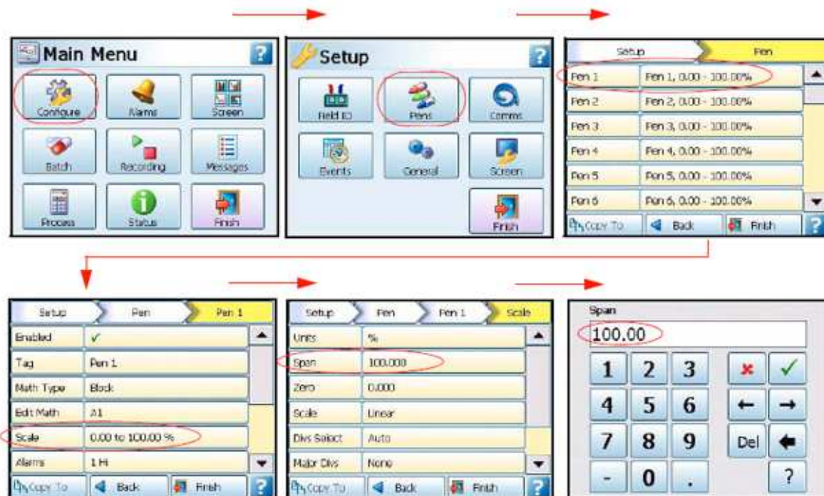
Example of a recorder menu path from the Main Menu to Pen Scale configuration with clear and rapid navigation
