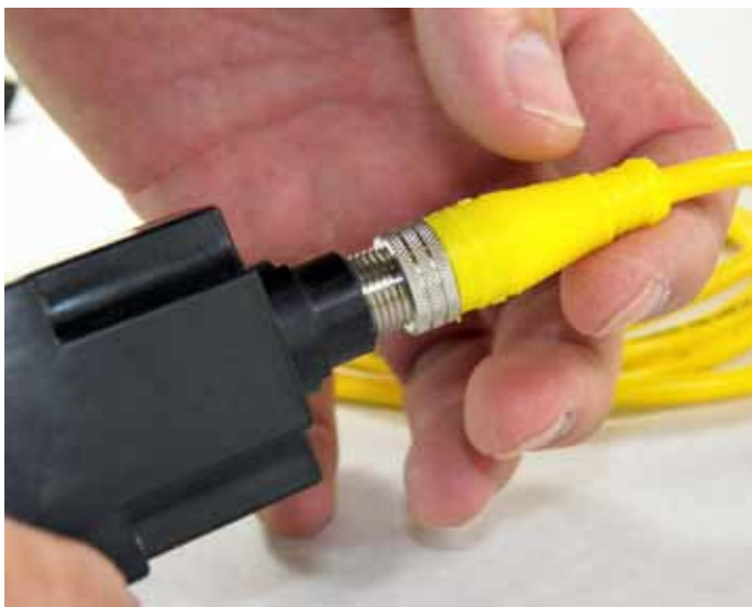
Figure 2. WLS Single Switch Adapter BT1 & BT2 Connector to Mate Cable
