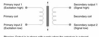
Phasing: Output is in phase with supply when the armature is outward of the electrical zero position
