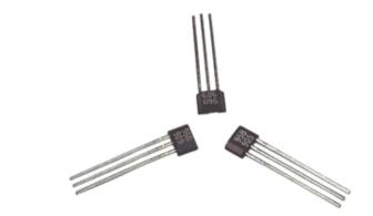
The SS490 Series MRL (Miniature Ratiometric Linear) sensors are small, versatile linear Hall effect devices which are operated by the magnetic field from a permanent magnet or an electromagnet. The ratiometric output voltage is set by the supply voltage and varies in proportion to the strength of the magnetic field.
