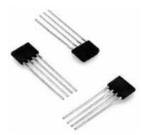
The SS42R Series is a Bipolar Latching Hall IC with a pair of complementary push/pull outputs. A dual Hall element is used to offset stress induced noise and drift. The operate and release points are laser trimmed to insure near-zero symmetry. The robust outputs are capable of sourcing up to 6.4 mA and sinking up to 4.4 mA. The device contains inherent reverse polarity protection up to the full power supply rating.
