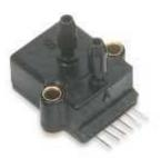
The SCX series sensors provide a very cost-effective solution for pressure applications that require operation over wide temperature range. These internally calibrated and temperature compensated sensors were specifically designed to provide an accurate and stable output over a 0 °C to 70 °C [32 °F to 158 °F] temperature range. This series is intended for use with non-corrosive, non-ionic working fluids such as air, dry gases and the like.
