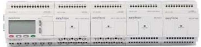
1.16 pcs extensions can be applied to the PR-18 or PR-24 CPU
