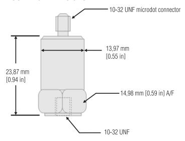
Model MAQ13 Accelerometer
