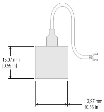
Model MA23 Accelerometer
