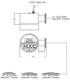
\*Models JPB, JPE, JPR, JPX, JPV No cable for battery powered Model JPW
