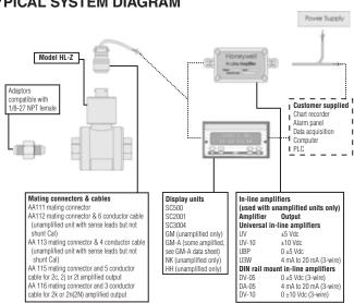
NOTE: For long cable runs or electronically noisy environments, an amplified sensor or locally mounted amplifier is often preferred.
