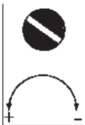
Direction of action of setting spindle
