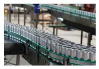
At an entire occupancy of the sensor-surface with tins a signal is released. If this is absent, the can line has a gap and the conveyor speed must be raised. Furthermore sensor strips are also available with the Teach-In function (without surcharge). This variant of the sensor recognises the available installation condition after the key is pressed and adjusts the operating distance optimally.
