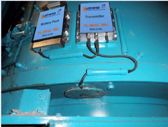
Installation of Transmitting unit and Changeable Battery Pack at a mixer drum
