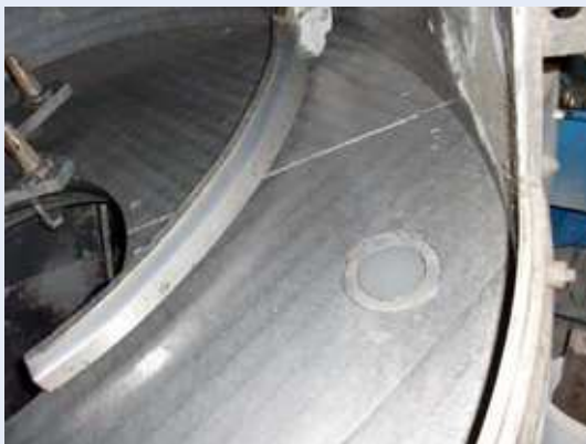
Probe installation in a rotating mixer floor
