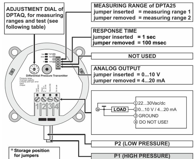
Fig. 3. Wiring details
