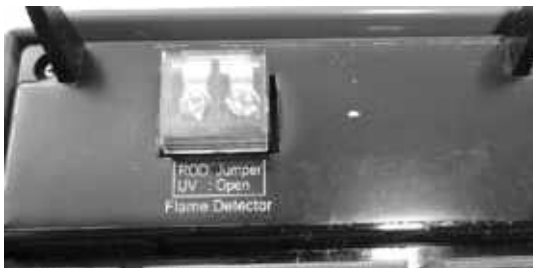
STD & ENH Models (flame detector select only)
