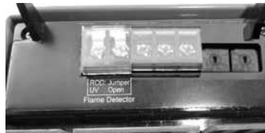
ULT Model (bus connector and address switches)
