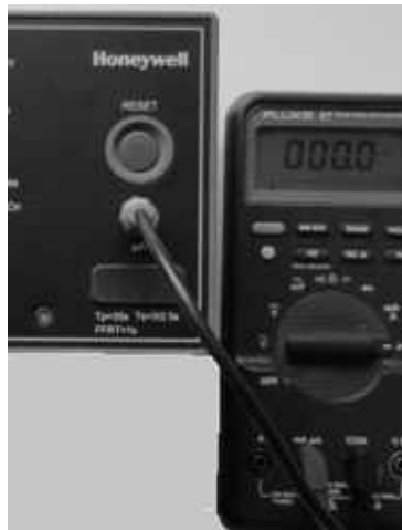
Fig. 4-3: Measuring flame signal with multi meter ( \mu\text{A} range selection) using a jack plug.
