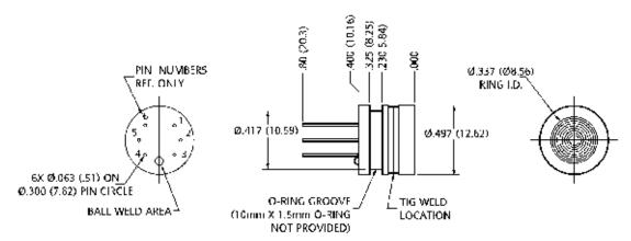
Note: Non-concentricity effects at the diaphragm weld area may cause runout of up to ±0.006 in between the upper and lower portions of the sensor body. (It is recommended to use a counter bore to mate with this device to allow for this nonconcentricity).
