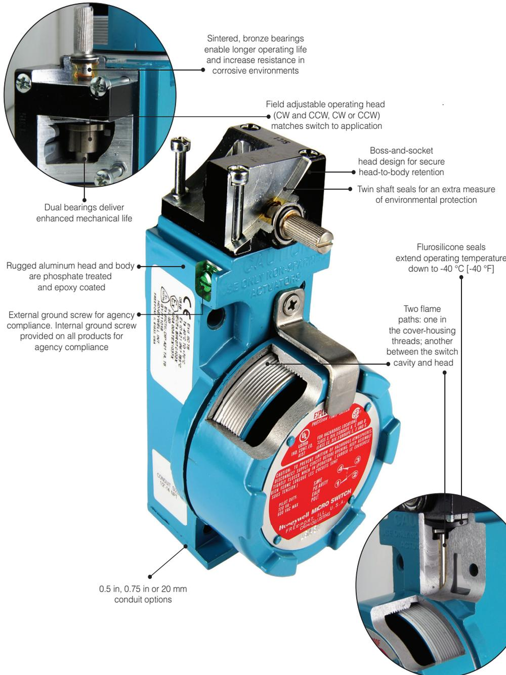
*Honeywell's MICRO SWITCH™ BX/BX2 Series of hazardous location limit switches can be used in hazardous or explosive environments around the globe. They offer a variety of options for actuators, housing materials, contacts, and sealings, as well as meet global certifications.*
