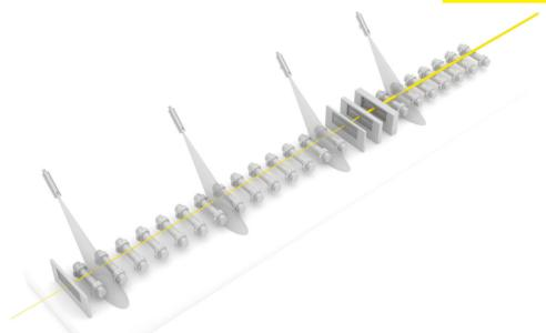
Infrared sensors to monitor material
