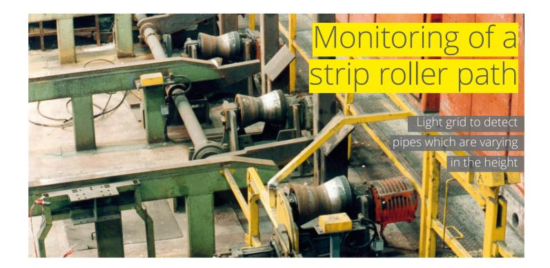
The exactness of the tube length measurement depends on the capability for reproduction to detect the tubes beginning and end. A tube rolling mill needed length measurement directly at the conveyor track of the subsequent production. An easy commissioning, high repeatability and an integrated error monitoring were in demand. As there are tubes of different sizes in process, they have decided on the Proxitron light grid.
