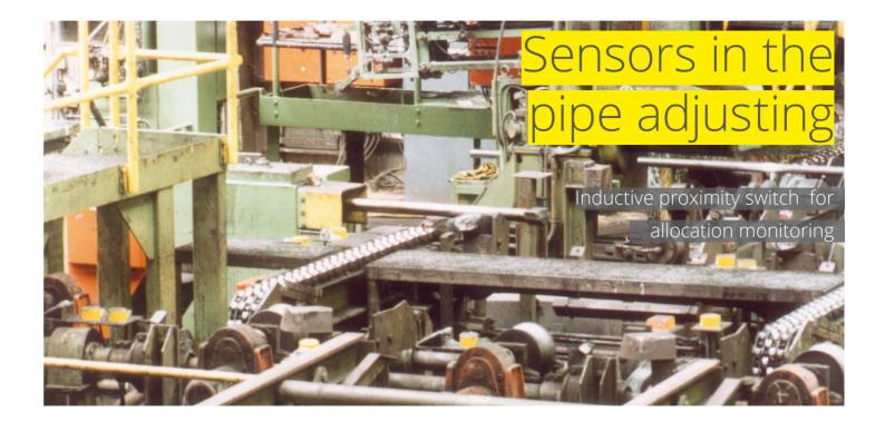
Sensors must be resistant and need to operate smoothly under harsh conditions in the industry. The sensors function cannot be affected by dust, steam, heat or cold. Proxitron inductive proximity switches meet these requirements, such as in the pipe adjusting in tube production.
