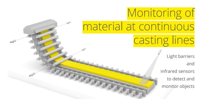
Continuous casting lines, block casting lines, and billet casting lines continuously deliver semi-finished products for further processing in the rolling train. Proxitron light barriers, Piros infrared sensors and pyrometers are ideally suited for material recognition and monitoring in the area of the cut-to-length line and recognition of the approaching piece.
