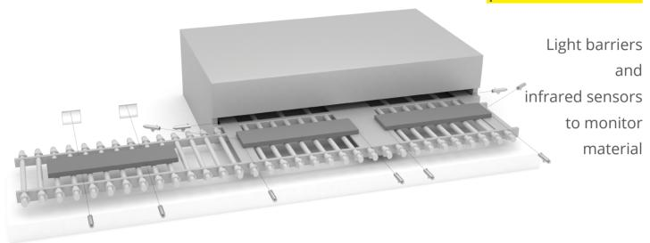
After the semi-finished material - e.g. a block - had been heated to the rolling temperature in a walking beam furnace, it is rolled to a defined measurement in the blooming train. This measurement is the tapping for the finishing train. Each end rolled product has its own tapping cross-section, which is related to the calibration, profile and individual passes on the rolls.
