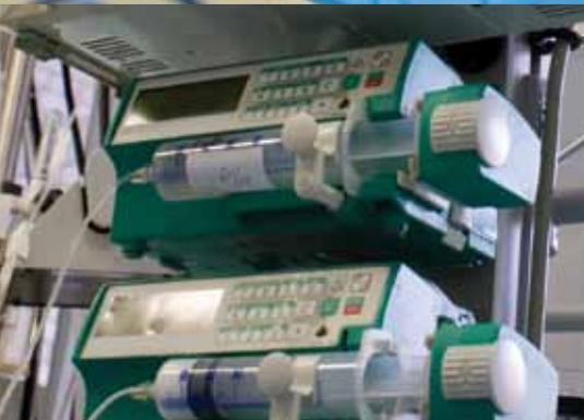
An infusion, insulin, or syringe pump—typically a screw pump that pushes on a syringe or cartridge—is used to deliver small amounts of medication to a patient intravenously.
